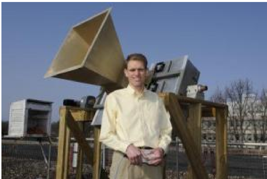
One of the instruments Brian Hornbuckle uses to measure soil moisture content is a microwave radiometer. (Credit: ISU photo by Bob Elbert)
